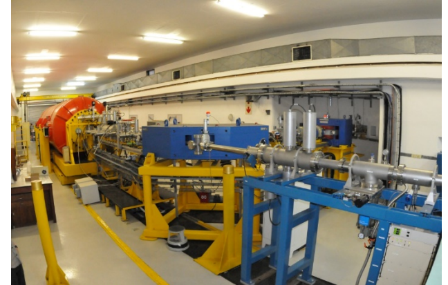
Fig. 2.15 Long-term erosion rate assessment work flow including a) sampling of river deposits (Photo: J. Baade 2019), b) preparation of targets for AMS measurements (Photo: C. Glotzbach 2020), c) determination of beryllium concentrations with an accelerator mass spectrometer (AMS), here the facility at iThemba LABS in Johannesburg (Photo: J. Baade 2015).
